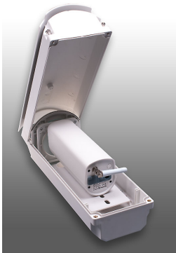
The EYE-02 mounted into Outdoor Cover with glass. EYE-02 body should touch front panel.
